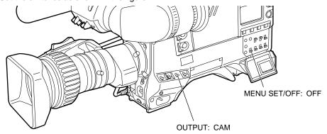
Press the AUTO W/B BAL switch to the ABB side and then release the switch. The switch returns to the center and the black balance is automatically adjusted.
